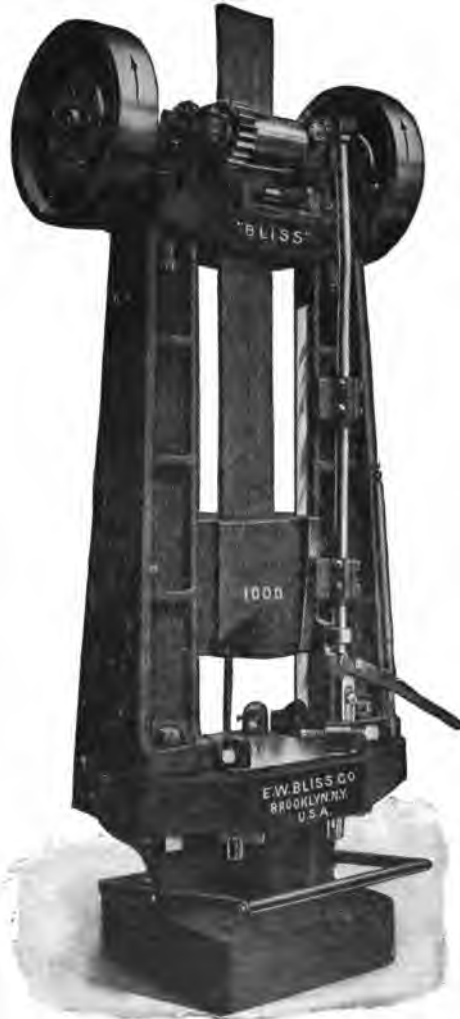
Fig. 19. Board Drop Hammer Courtesy of E. W. Bliss Company, Brooklyn, New York
